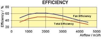
The efficiency concerns the fan without a motor.
