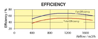
The efficiency concerns the fan without a motor.
