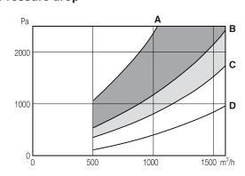
The pressure drop across FilterBox varies with air flow and dust load. Maintaining a certain average air flow with increasing dust load requires a shorter interval between cleanings.
