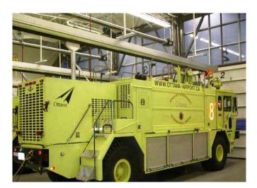
Vertical Stack is a fully automatic exhaust extraction system for vehicles with top exhaust pipes. The vehicle either drives backwards into the parking bay or drives through.
