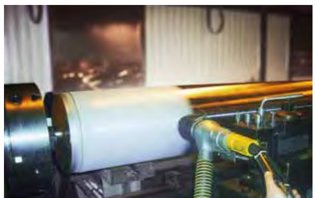
Removes paint, rubber/plastic coverings on floors, rollers, etc. to give a new surface coating good adhesion
