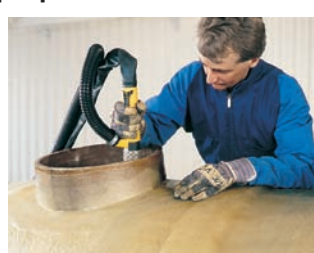
On-tool trimming composites
