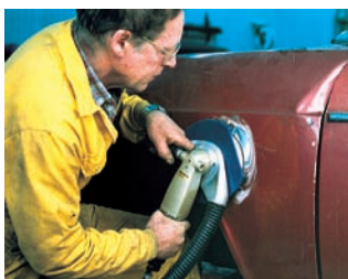
On-tool extraction of sanding dust
