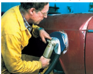
On-tool extraction of sanding dust
